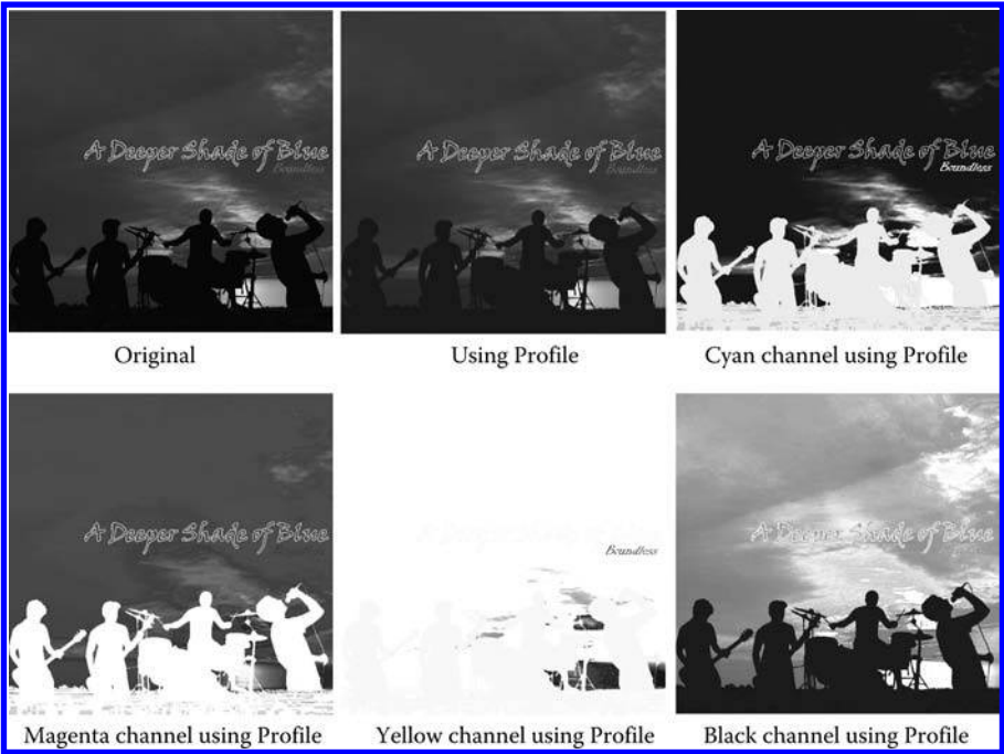
FIGURE 28.24 Image simulation for Profile #2 with constrained GCR inverse LUT.
