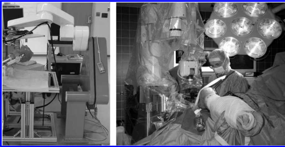
FIGURE 20.1 The NEUROMATE neurosurgical robot (left) and the ROBODOC hip replacement system in clinical use (right). (Courtesy of Peter Kazanzides).
