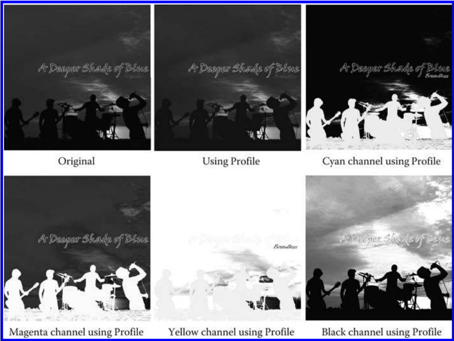
FIGURE 28.23 Image simulation for Profile #1 with constrained GCR inverse LUT.
