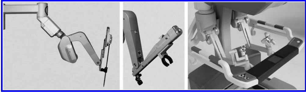
FIGURE 20.2 The da Vinci Surgical System includes multiple instrument (left) manipulators, an endoscopic camera-holding (middle) slave manipulator, and a console containing a stereo video viewer and master manipulators (right). (Copyright Intuitive Surgical, Inc.).
