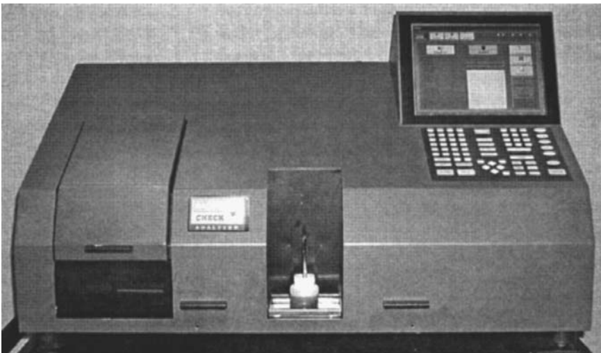
FIGURE 22.6 Integrated oil analyzer for engine and oil condition monitoring. (From Practicing Oil Analysis 2001, Conference Proceedings, Noria Corp., Tulsa, Okla. )
