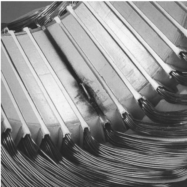
FIGURE 8.14 Winding grounded in the slot.
