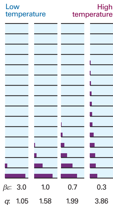
Fig. 16.6 The populations of the energy levels of the system shown in Fig. 16.3 at different temperatures, and the corresponding values of the partition function calculated in Example 16.2. Note that \beta = 1/kT .
