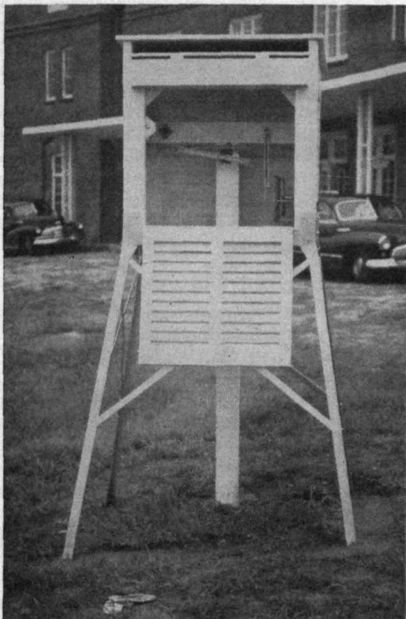
FIG. 2-4. Instrument shelter with maximum and minimum thermometers and psychrometer. (U.S. Weather Bureau.)
