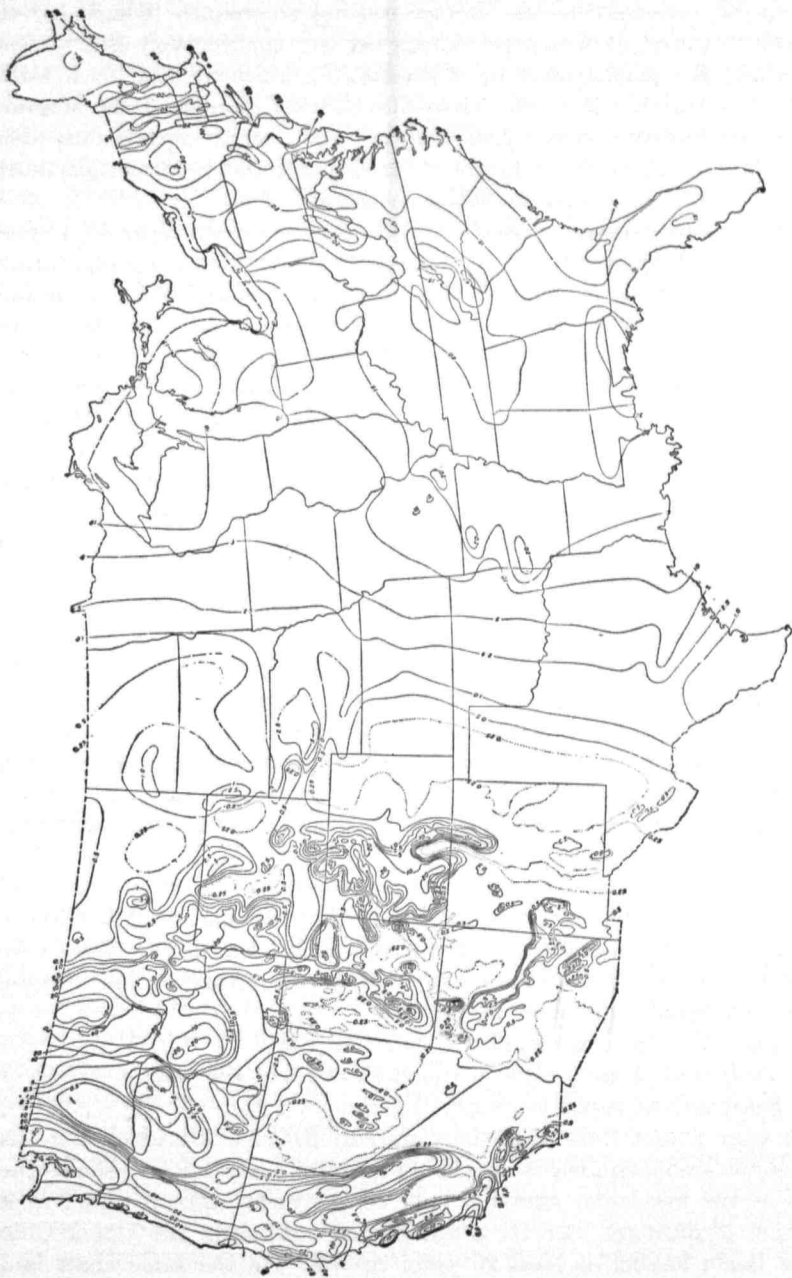
FIG. 4-21. Normal annual runoff in the United States. (U.S. Geological Survey.)
